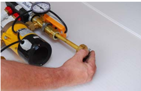
Step 4: remove entire immersion sleeve
