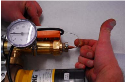
Step 13: ...with attention to soldered joint between tube and sensor (stainless fitting)
