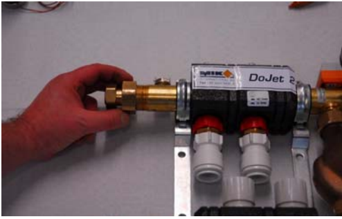
Step 8: Assemble new flange socket with seal
