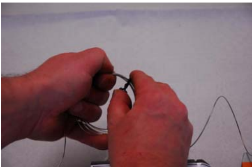
Step 12: Carefully put sensor tube in order and fasten with plastic clip...
