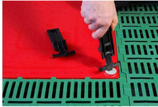
2. open locking screw with included tool
