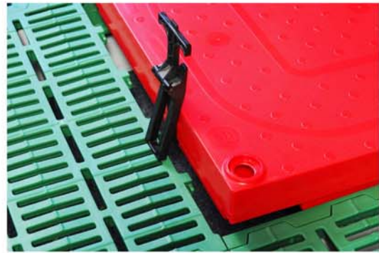
4. use tool as pedestal holding up the panel
